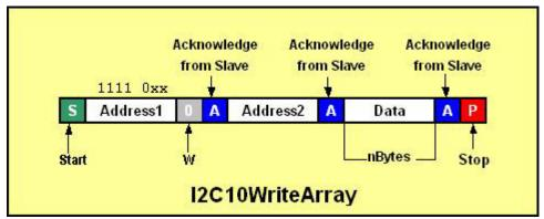
The DLL is currently set to write up to a maximum of 256 data bytes (nBytes) in one I2C10WriteArray transmission.
