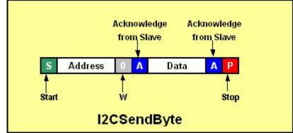
device address and one data byte. I2CSendByte returns any error condition it encounters. The function ensures that the least significant bit of the address is a '0' before it is sent to the target device.
