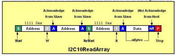
proper 10-bit I<sup>2</sup>C compliant format. A subaddress is also sent after the second byte of the address (not shown in diagram below).
