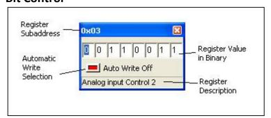
The Bit Control is activated when the user presses the Bit Control button on the User Defined Device screen or by right clicking the grid and then selecting 'Use Bit Control to Change Active Register' from the pop-up menu.
