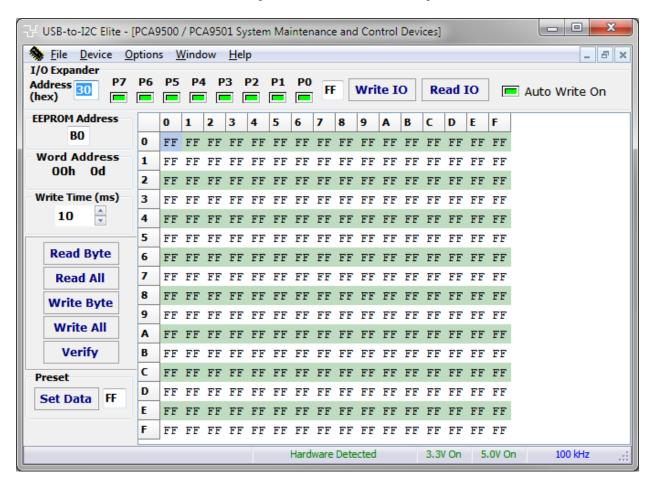
The PCA9500 and PCA9501 are 8-bit I/O expanders with an on-board 2-kbit EEPROM. The eight quasi bidirectional data pins can be independently used as inputs or outputs to monitor board level status or activate indicator devices such as LEDs. The data for each Input or Output is kept in the corresponding Input or Output register. The system master can read all registers.
